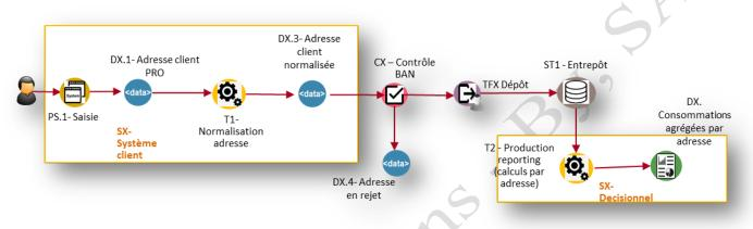
This chain describes the succession of processing stages, from entering an address to its use, to provide aggregate measurements by address.
