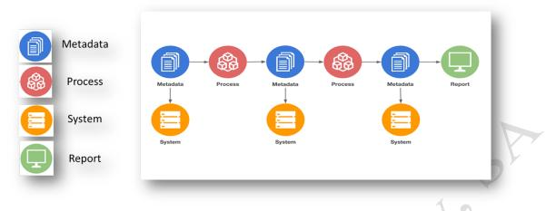
Data lineage consists in providing the processing chain that allows the regulatory report to be produced, by identifying the systems (example: a database) and processes (activities: data processing – examples an ETL script, an algorithm) concurrent to producing the report and by highlighting the information about the data (metadata: column name in a table for example).
