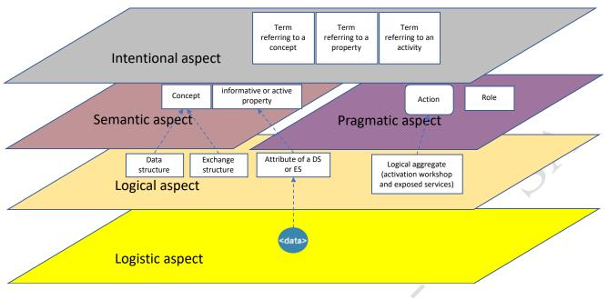
Figure PCD-64\_13. The types of elements manipulated in the action "Locate data"
