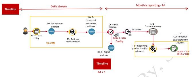
On this diagram, the execution metadata is in red: execution time, data quality obtained – example: address quality, instance and version of a report that is the focus of data lineage...
