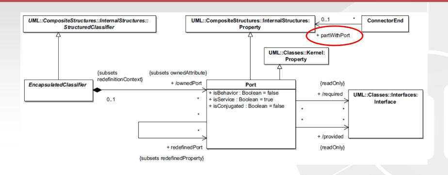
If a connector end references a *partWithPort, then the role must be a port that is defined by the type of the partWithPort.*
